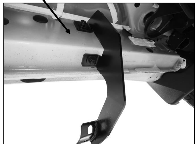
(Fig 4) Driver/left front Bracket installed
