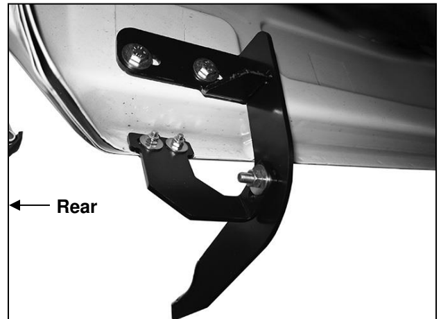
(Fig 18) Driver/Left rear Mounting Bracket assembly
