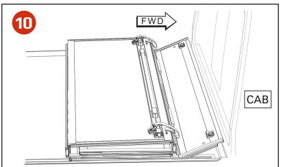
The small panel faces forward, toward the cab and folds down over the slotted rail brackets. The front panel must sit just inside the bulkhead rail with the seal resting on top of the bulkhead. Fold the panel down and align it so it is setting squarely on the rails and align the mounting holes with the slotted rail brackets.
