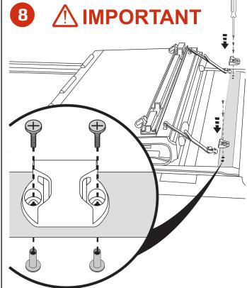
Before placing the cover on the truck, use a screwdriver to install the two buckle ends into the pre-drilled holes on the front header panel with the provided machine screws and threaded posts
