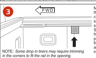
Make sure the rail is clamped square as shown.
