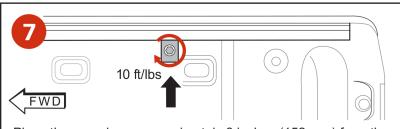
Place the rear clamp approximately 6 inches (152 mm) from the tailgate. Tighten all of the clamps until snug. Then torque an additional 1/2 turn, (10 ft-lbs).
