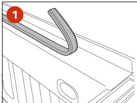
If the truck does not have a drop in bedliner, install the cab/bulkhead seal (weather strip). Wipe paint ed surface with isopropyl alchol before applying. If the truck has a drop in bedliner, no seal will be needed.
